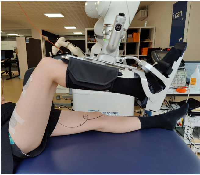
Figure 1: ROBERT® is a seven-degree-of-freedom robotic manipulator that can move the lower limb of a patient in a lying position. The participant's leg was attached to the end effector of ROBERT® through a foot brace.
