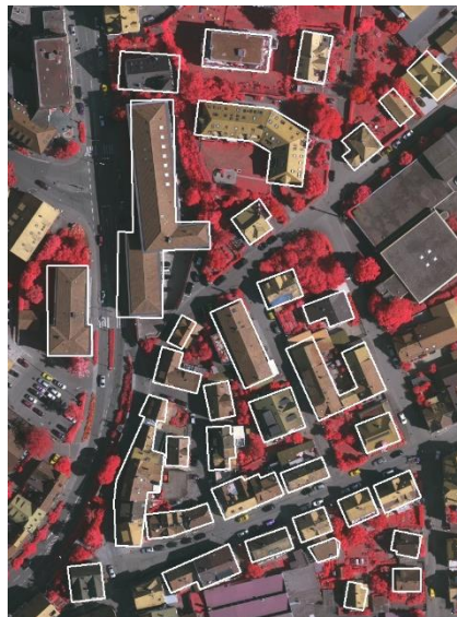
Figure 18: Enhanced outlines of buildings plotted on top of an DSM-based orthoimage. (Source: Höhle, 2021)
