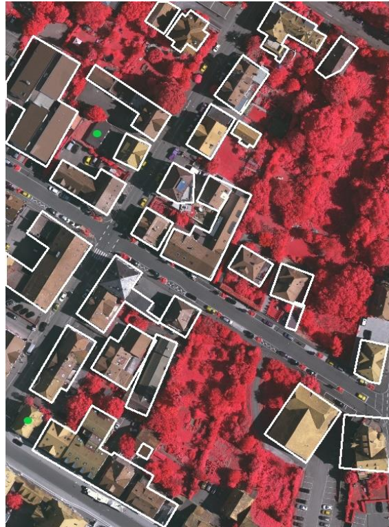
Figure 24: Enhanced vector data of building outlines superimposed onto the DSM-based orthoimage. The green dots indicate undetected buildings. (Source: Hhle, 2021)
