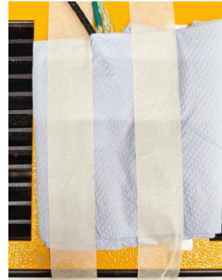
Figure 27. Calibration well with thermometer probe and thermocouples.
