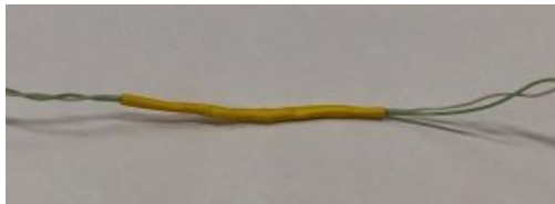
Figure 49. The finished connection between two thermocouples.
