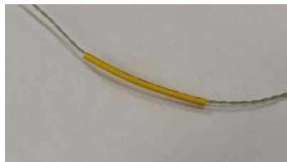
Figure 46. Shrinkable tubing on one of the thermocouples.
