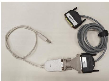
Figure 15. Helios data-cable connected to an USB-to-serial converter.
