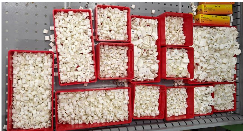
Figure 43. Cable marking for thick thermocouples.
