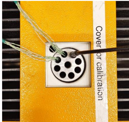
Figure 27. Calibration well with thermometer probe and thermocouples.
