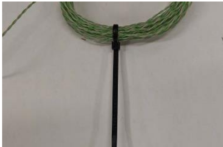
Figure 39. Gathering of free hanging thermocouples with zip tie.
