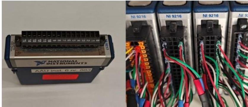
Figure 31. Different NI modules used for RTD measurements.
