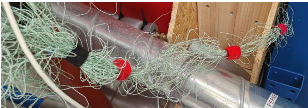
Figure 38. Gathering of free hanging thermocouples with Velcro.
