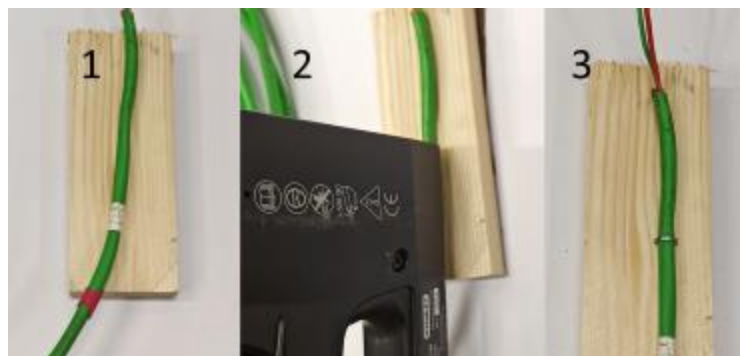
Figure 36. How to mount thick thermocouples on flat surfaces.
