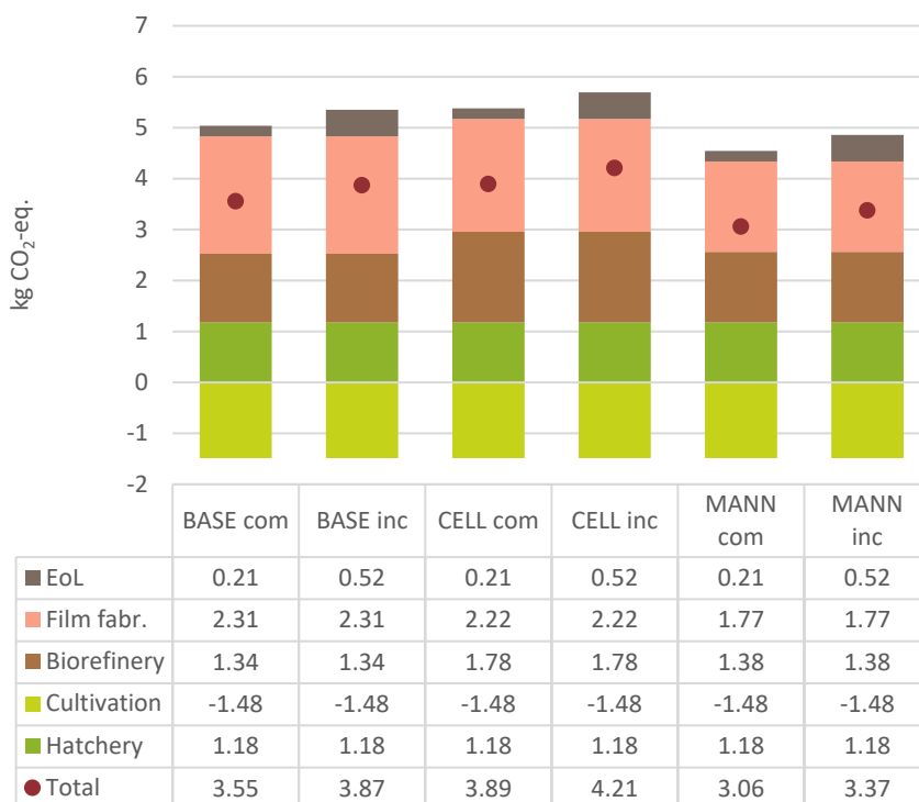
Figure 4-4: Impacts in the global warming category accounting for the biogenic carbon based on the scenarios.
