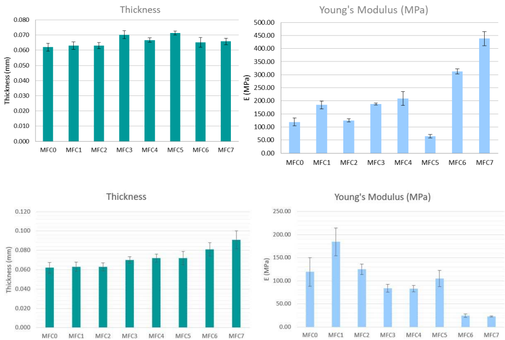
Figure 10: Effect of MFC cellulose on film properties with (top) and without (bottom) thickness control.
