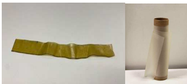
Figure 8: Seaweed based films fabricated with alginate from the biorefinery (SINTEF, left) and highly refined commercial alginates (Algaia, right).
