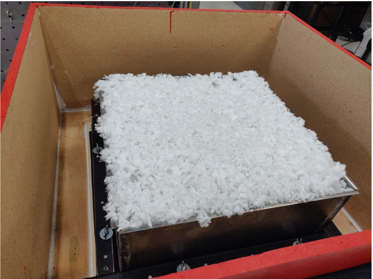
Figure 20: Loose-fill blown glass wool test sample in sample holder metal frame of the air permeameter.
