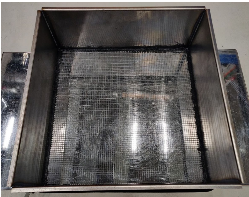
Figure 7: Sample holder metal frame without any test sample.
