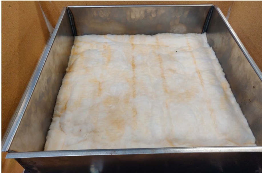
Figure 13: Test sample (glass wool mat) inserted in the sample holder metal frame.
