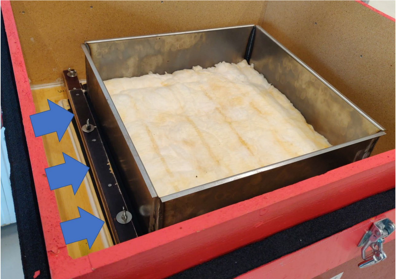
Figure 16: Push on the sealing bars and tighten the tightening screws on each of the 4 sides of the sample holder metal frame.
