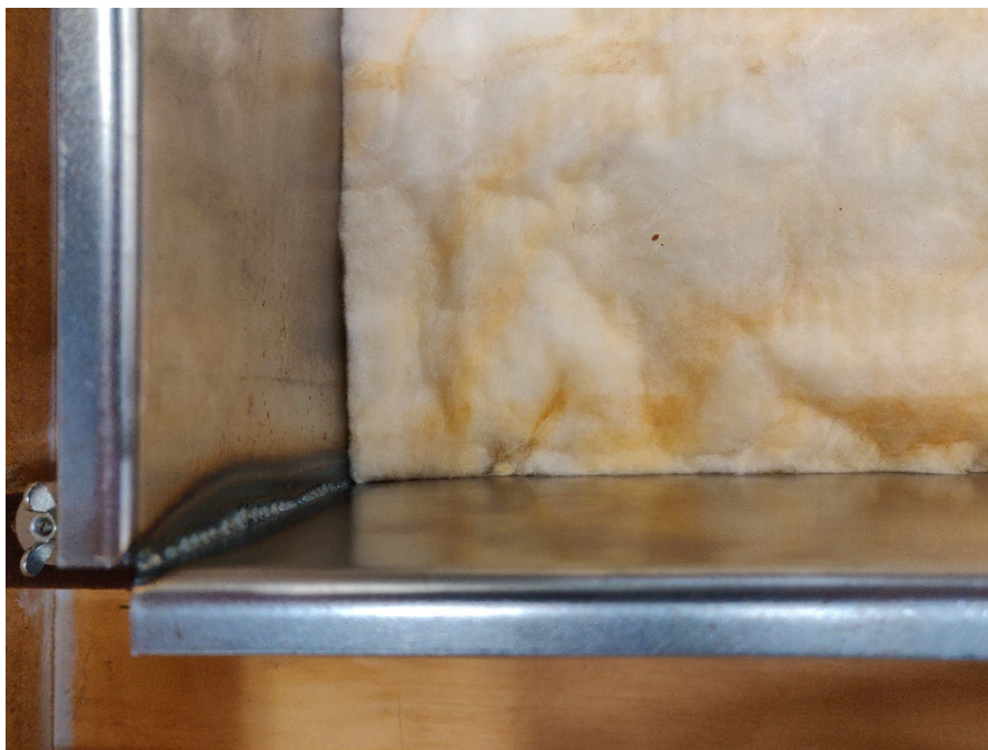
Figure 14: Ensuring no air gap between the test sample and the sample holder metal frame.
