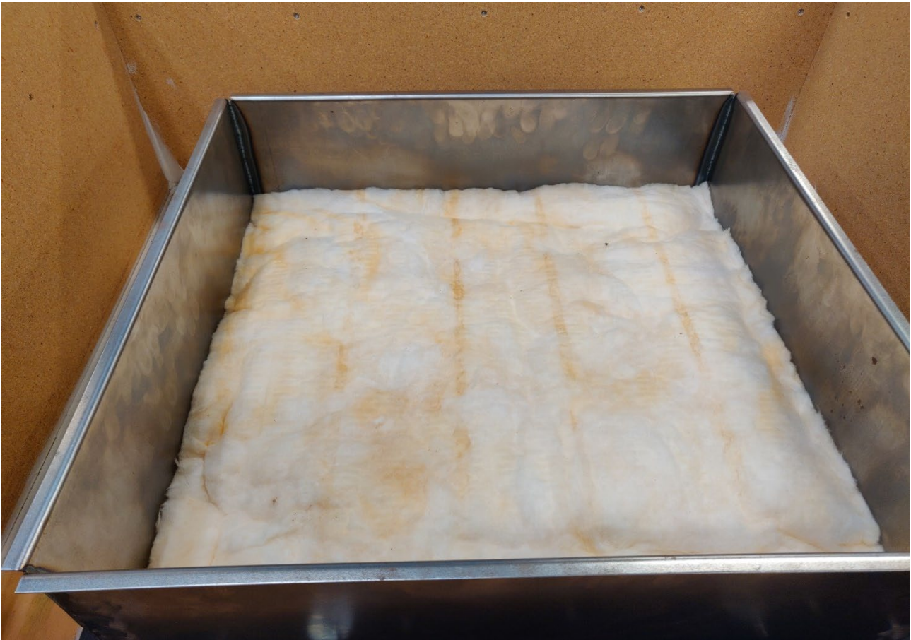
Figure 17: Glass wool mat test sample in sample holder metal frame of the air permeameter.
