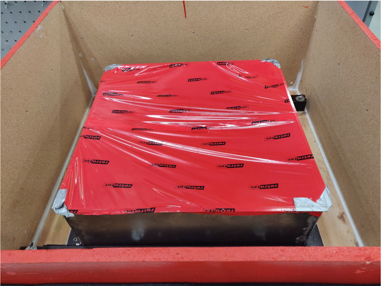
Figure 11: Sealing of the top side of the sample holder metal frame for the air leakage test of the entire air permeameter.
