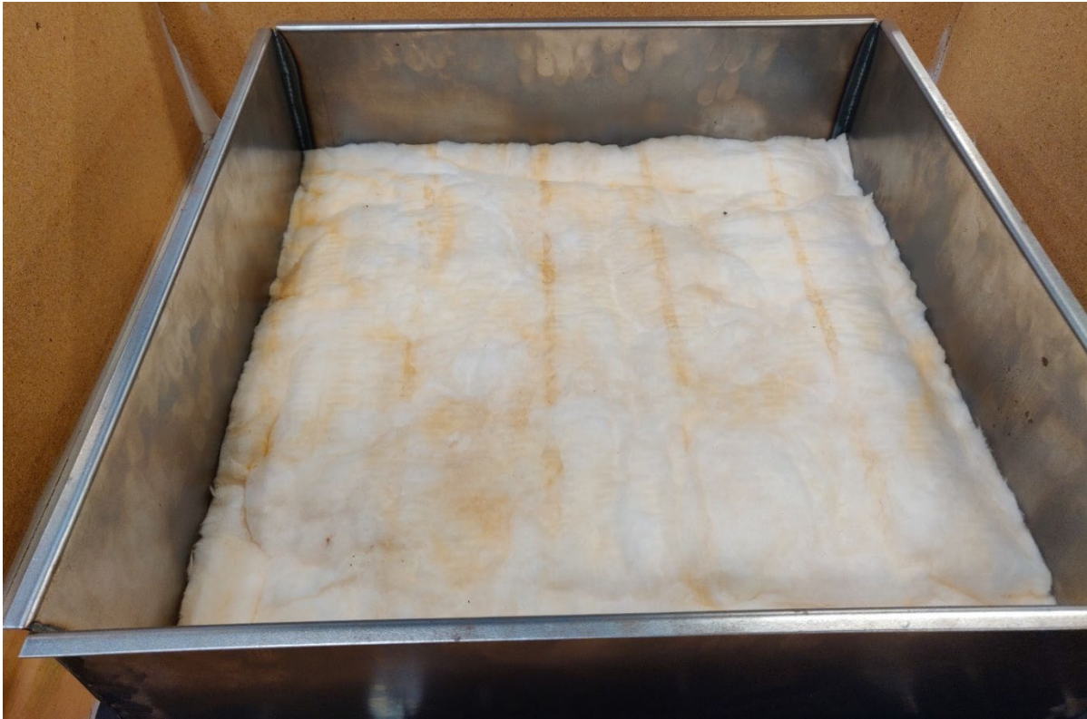
Figure 6: Test sample (glass wool mat) inserted in the sample holder metal frame.
