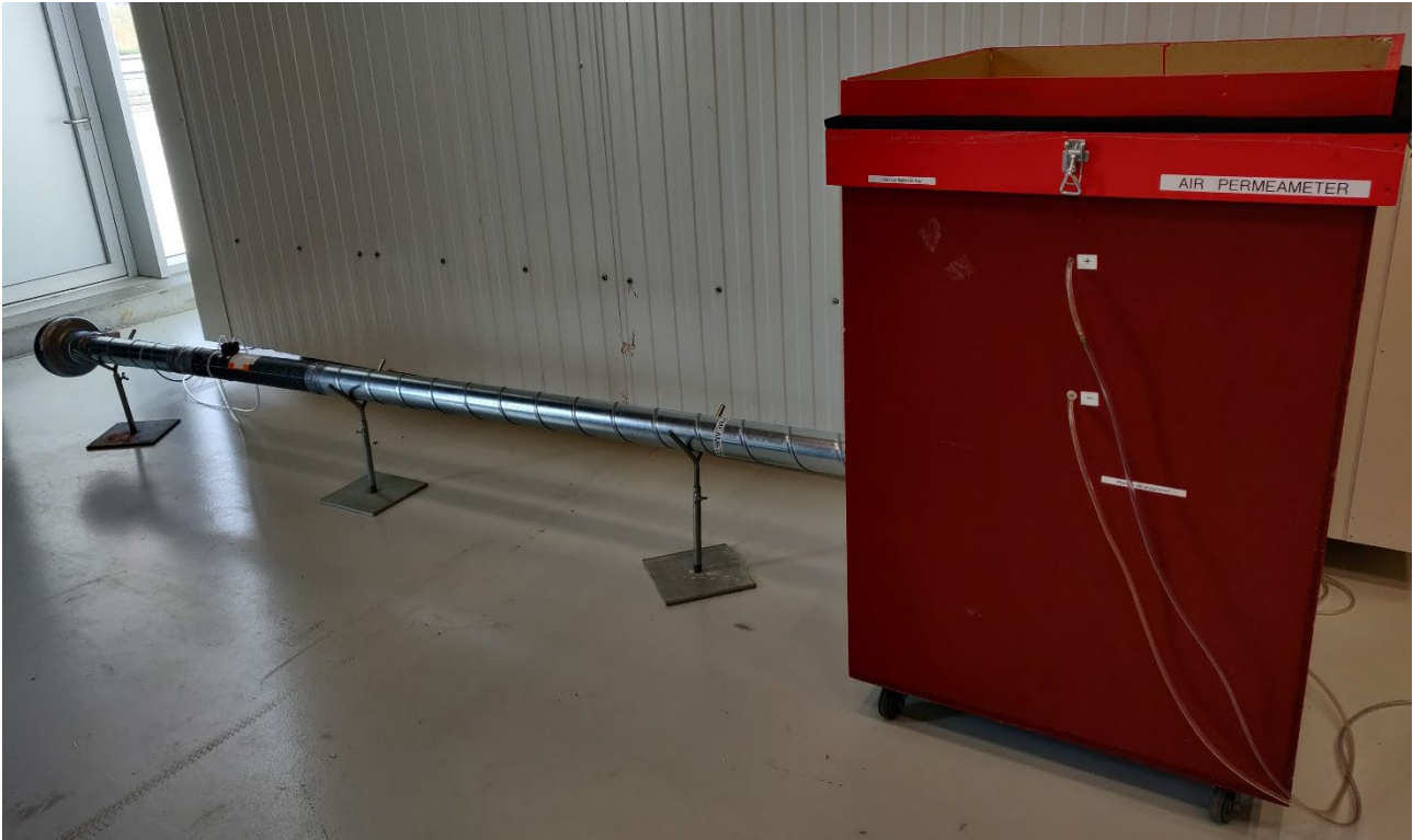
Figure 2: Overview of the experimental setup for measuring the effective air permeability.
