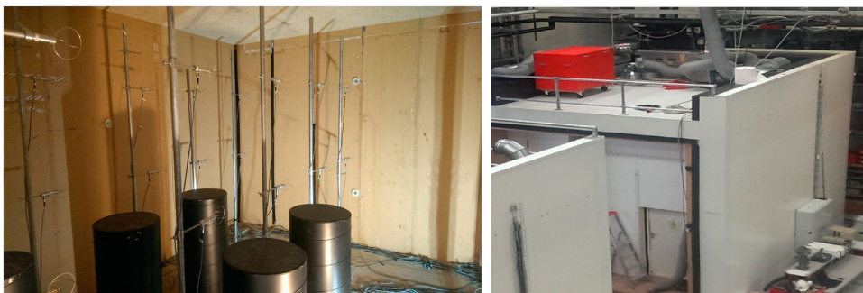
Figure 1. Inside (Rahnama et al., 2020) and outside view of the guarded hot box located at Aalborg University, Department of the Build Environment.
