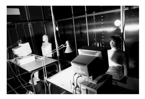
The test room is the IEA Annex 20 room with length, width and height equal to 4.2 m, 3.6 m and 2.5 m.
