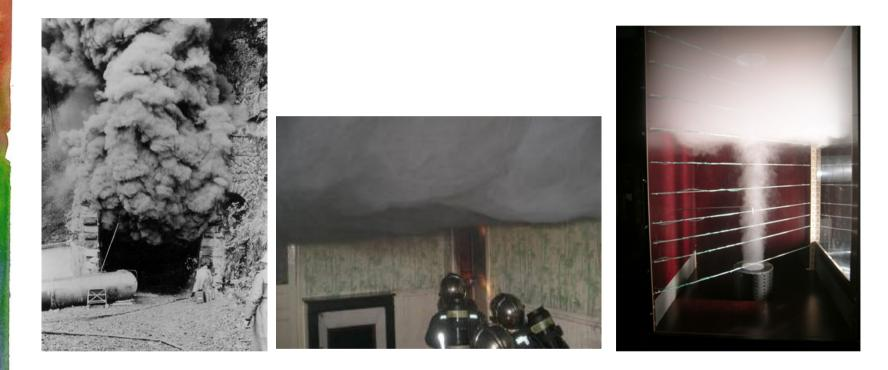
Hot smoke will normally produce an upper zone in a space With a fire.
