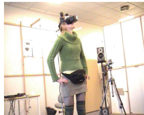
FIGURE 3: A subject navigating in the virtual environment wearing a head-mounted display (HMD).
