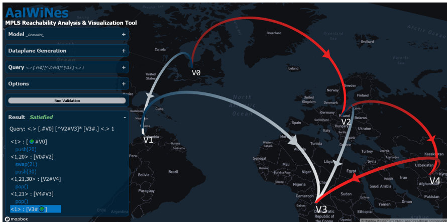
Fig. 7: The graphical user interface of AalWiNes showing the result of a longest trace query on a small example network.
