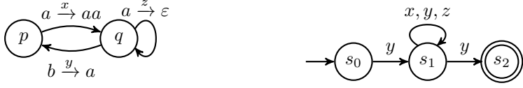
(a) PDA \mathcal{P}_1 where rules are arrows between control locations annotated with stack modification and rule label (b) NFA \mathcal{A}_1 for the regular expression y(x|y|z)^*y
