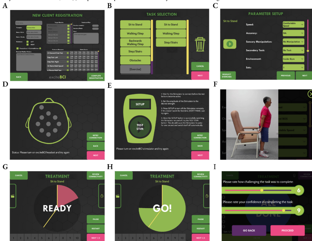
Figure 3. Example screenshots from the exciteBCI app interface prototype v3.3. (A) Registering a new patient, (B) the task selection suite where the patient and therapist select tasks that align with the patient’s goals, (C) the parameters that can be manipulated for each task by the therapist to ensure an optimal level of task difficulty, (D) checking the impedance levels of the electroencephalography headset, (E) the muscle stimulator is connected to the app and stimulation amplitude saved, (F) the patient watches a video on how to perform the task, (G-H) the timing signal (auditory-visual cue) to get ready and execute the task, and (I) the patient completes the task difficulty and confidence ratings at the end of the task set.
