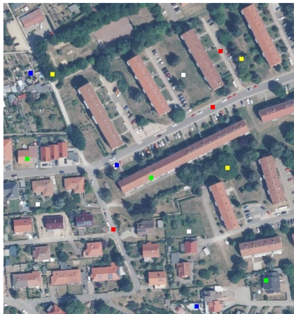
Figure 1. DSM-based orthoimage and samples of the selected classes (green: ‘building’, red: ‘impervious surface’: white: ‘low vegetation’, yellow: ‘tree’, black: ‘clutter background’).
