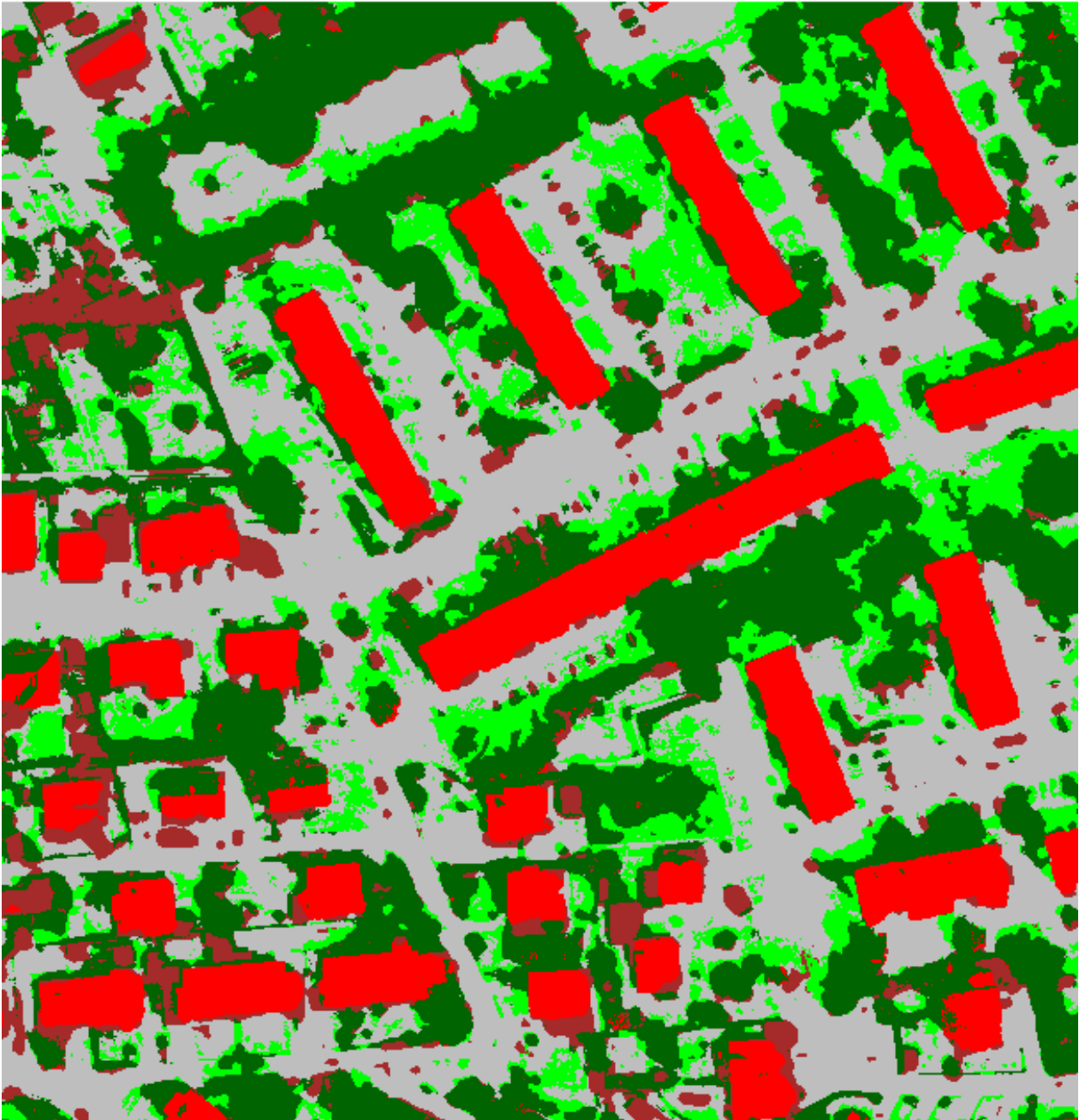
Figure 3. Generated land cover map (red: 'building', gray: 'impervious surface', green: 'low vegetation', dark green: 'tree', brown: 'clutter background').
