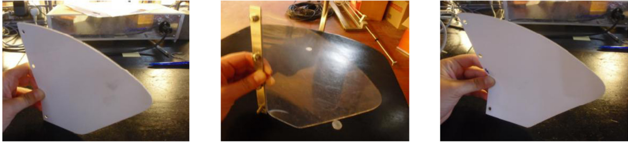
Figure 9. The three thicknesses tested. From the left: 1mm, 0.75 mm and 0.4 mm thickness.
