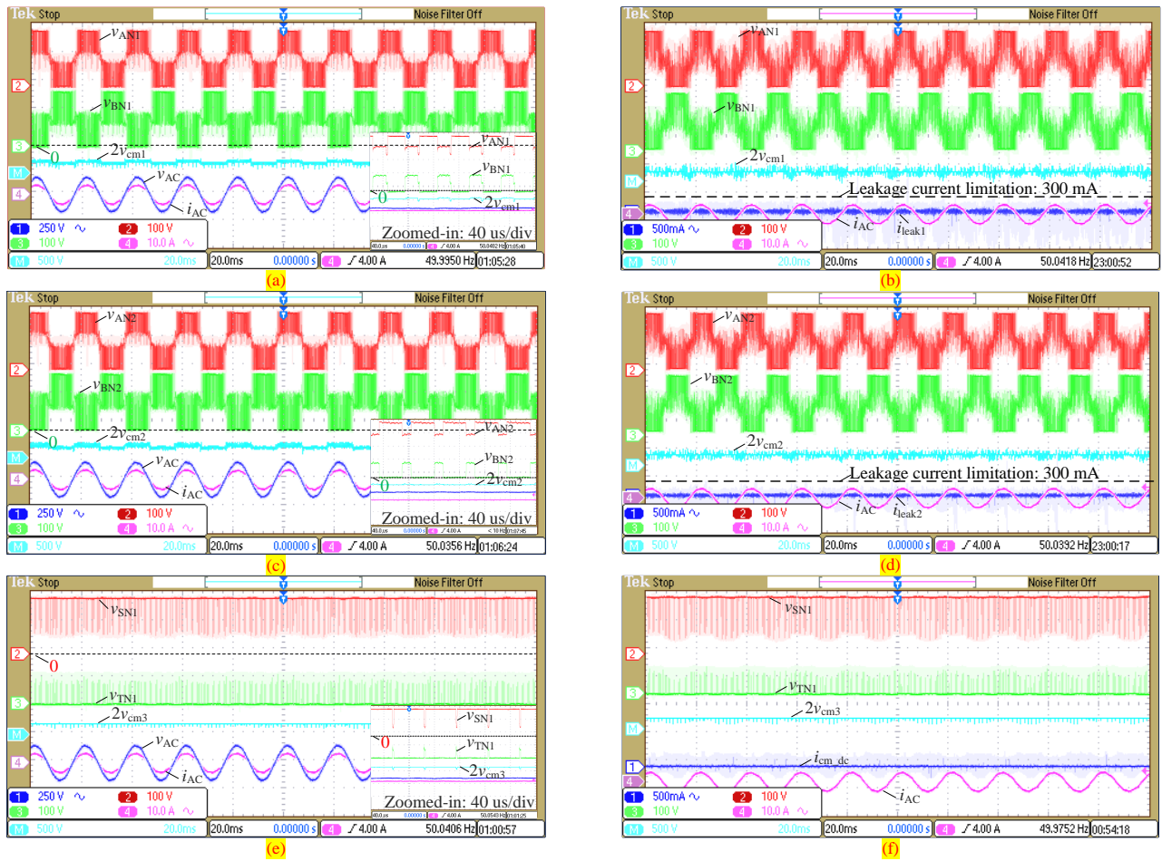
Fig. 13. CM performance of the proposed hybrid converter, (a) v_{cm1} , (b) i_{leak1} , (c) v_{cm2} , (d) i_{leak2} , (e) v_{cm3} , and (f) i_{cm\_dc} (time: 20 ms/div).
