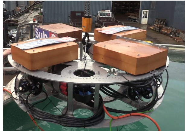
Fig. 5. UUV Prototype cleaning robot, note the placement of the vertical thrusters represents a previous design change.
