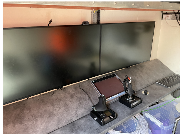
Fig. 6. Topside control system with pilot joystick.
