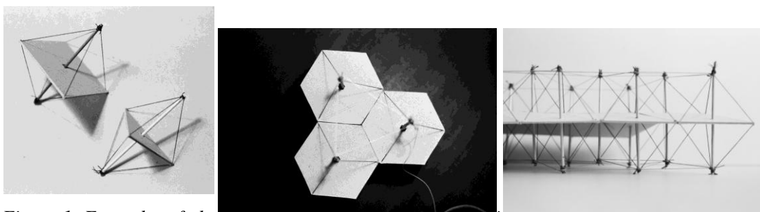
Figure 1: Examples of plate tensegrity units; different plate simplex types (left and centre) and a side view of an assembly showing the middle platelayer inscribed by cable-nets (right).
