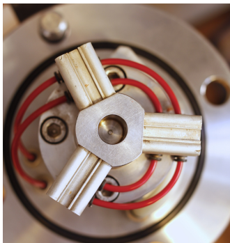
Figure 3.14: Locking mechanism in the load cell set to open.
