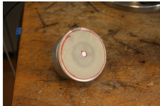
Figure 3.4: Rubber membrane rings mounted onto the pressure head with grease in between.
