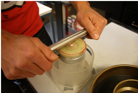
Figure 3.3: Steel rod squeezes out the air bobbles and distributes the grease evenly.
