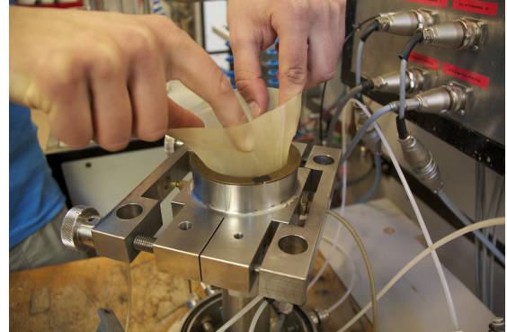
Figure 3.6: Wrapping the membrane over the sand form and brass ring.
