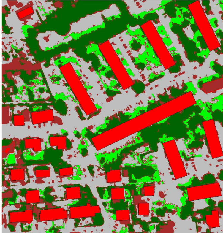
Figure 5. Enhanced land cover map: ‘buildings’ (red), ‘impervious surface’ (grey), ‘low vegetation’ (green), ‘tree’ (dark green) and ‘clutter/background’ (brown).
