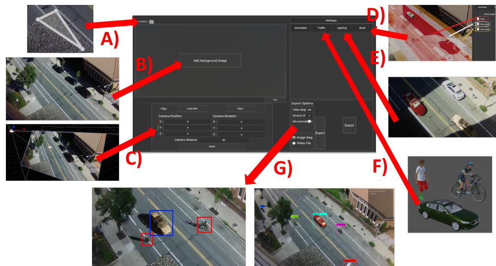
Figure 1. Overview of the pipeline built into the proposed application for synthetic augmentation of anomaly detection datasets through the use of the Unity game engine. The main aspects of the proposed solution are the user-centered menu system consisting of selecting occlusion parts A), loading images B), calculating the 3D position of the camera C), selecting roads D), adjusting the lighting and shadows of the scene E), and spawning 3D objects for normal and abnormal scenarios F), exporting the synthesized content G). The blue and red squares represent normal and abnormal objects, while the multicolored squares represent the different classes like cars, bicycles, and pedestrians.
