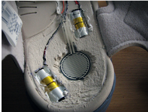
Fig. 1. Placement of a pressure sensor and two actuators in the heel of one sandal
