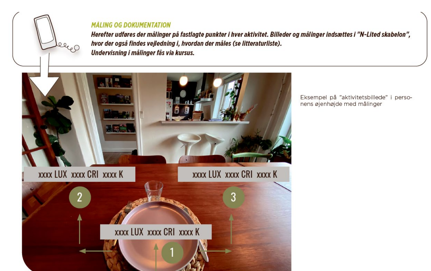
Example of an “activity photo” taken from the participant’s point of view, with measurements. From the N-Lited Manual [3].
