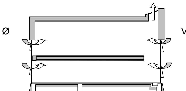
Figur 4. Princip for naturlig ventilation.
