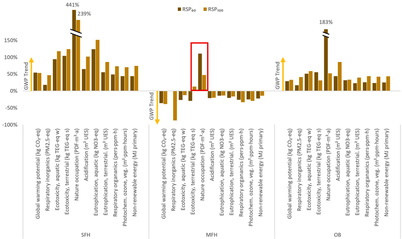
Fig. 4. The difference in impact between the conventional and wood-based scenarios (wood – conventional) for the considered impact categories for the three building typologies for RSP 60 and RSP 100 . The arrows show the GWP trend, and the red box highlights the impact categories that do not follow the GWP trend. Pay attention to the change in vertical axis values. SFH = single-family houses, MFH = multifamily houses, OB = office buildings. RSP 60 = reference study period of 60 years, RSP 100 = reference study period of 100 years, Photochem. ozone, veg. = photochemical ozone – vegetation, PM = particulate matter, TEG = triethylene glycol, PDF = potentially disappeared fractions of species, UES = unprotected eco-system, ppm = part per million, w = water, s = soil, m 2 -a = m 2 arable land.
