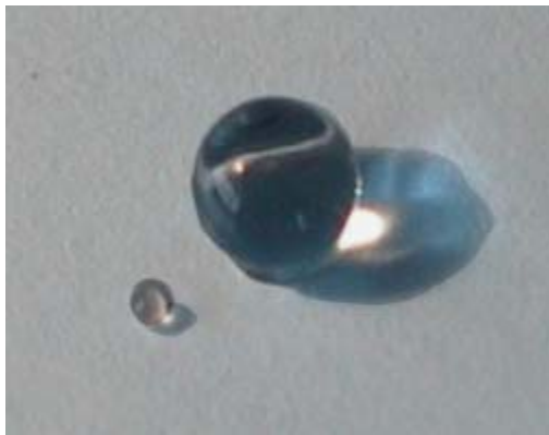
Figure 1. Superabsorbent polymers are swellable substances which can absorb many times their own weight of liquids by forming a gel. The absorbed liquid is not released even under moderate pressure [28]. The picture shows a dry, collapsed and a swollen suspension polymerized SAP particle.
