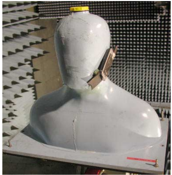
Figure 1. A handset mounted on the head/shoulder phantom.
