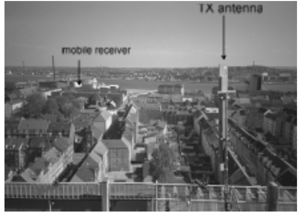
Figure 2 Picture of the transmitting BS antenna (the antenna is vertically mounted) and the view of the used urban area.
