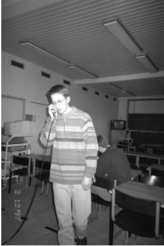
Figure 1 One of the test persons holding the handheld in what he feels as natural speaking position during measurement.
