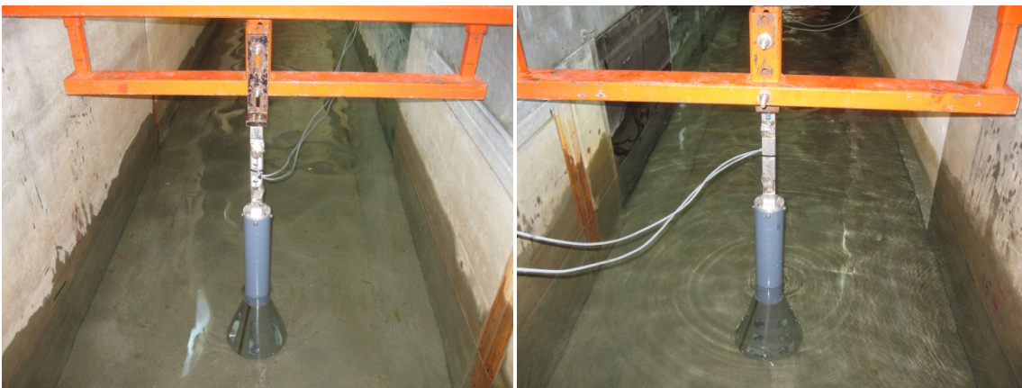
Figure 4. Positioning of the models TP6 (to the left) and TP7 (to the right) regarding the waves during the experiments.
