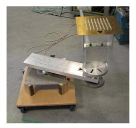
Fig. 1. The pedestal for circular movement of the transmitter array including the  $4 \times 4$  planar array of monopole elements with dummy elements. The element spacing is 2.5 cm.
