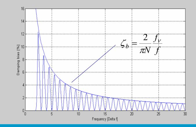
The absolute error on the damping in % (damping bias) as a function of the dimensionless frequency  $\alpha = f / \Delta f$
