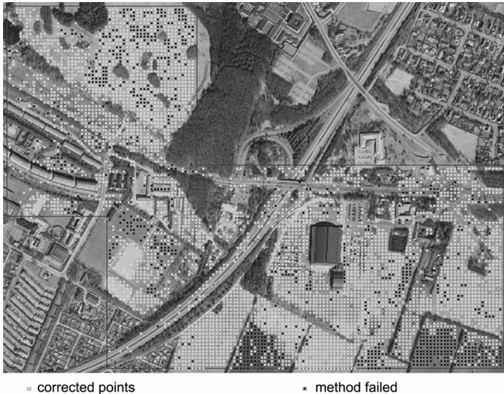
Figure 5. Division of the tested DTM into two categories, example of test B, sub area A_I. The white points fulfilled all set criteria and are corrected; dark points must be checked by other methods. The distance between the grid posts is 10 m. (Source: Potuckova, M., 2006)
