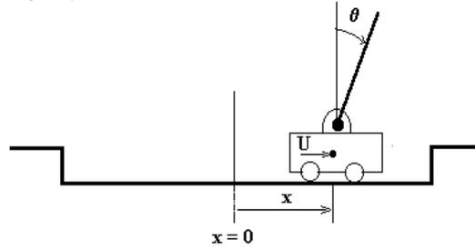
Fig. 2. Schematic diagram of the cart-pole syste
