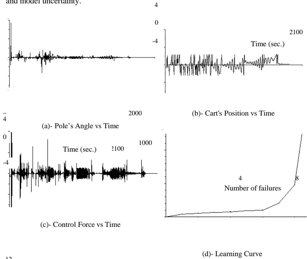
Fig. 7. Simulation results for  $l=0.5$ ,  $m=0.1$ ,  $m_1=2.0$
