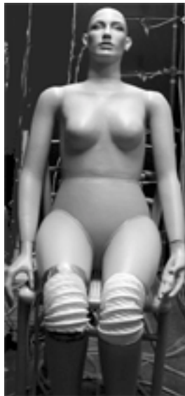
Figure 3. The full-scale Thermal Manikin Comfortina used in the heat loss measurements at Aalborg University
