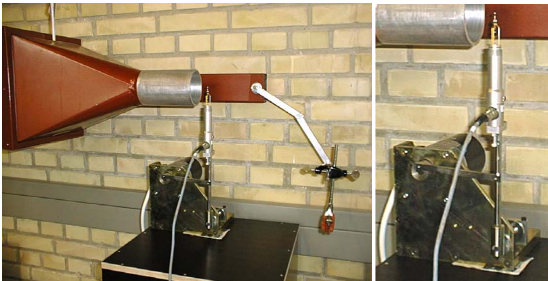
Figure 2. Picture of the experimental setup. When measuring, the anemometer is shielded from the surroundings by a Perspex tube (not shown in the picture).
