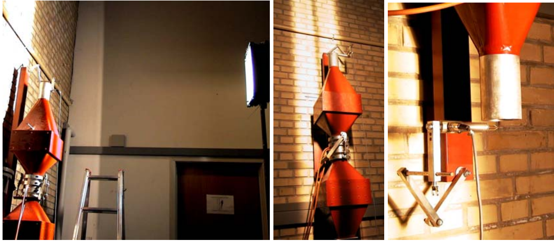
Figure 4. Hot-sphere anemometer in the jet-wind tunnel lit by the lamp imitating solar radiation.
