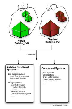
Figure 4 The Virtual Building (VB) model should be a digital copy of the real building, the physical building (PB), even before it is built.
