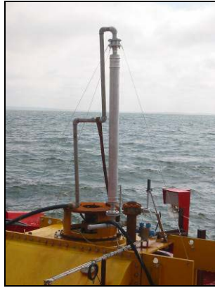
Fig. 4.2 Large diameter pipe installed in aeration tube
