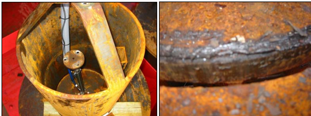
Fig. 4.5 Dummy turbine condition (31.03.03) and severe erosion of dummy turbine gate (11.08.03)
