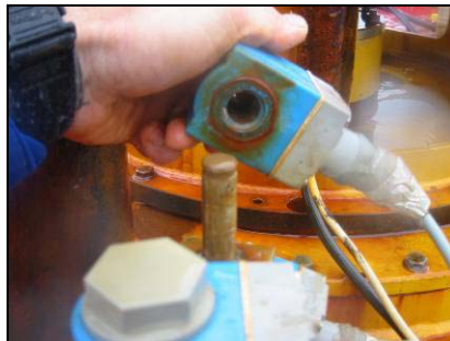
Fig. 4.4 Saltwater corrosion of solenoid (23.06.03)
