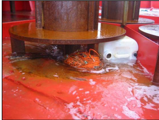
Fig. 4.3 Debris collecting at the dummy turbine cylinder gate
