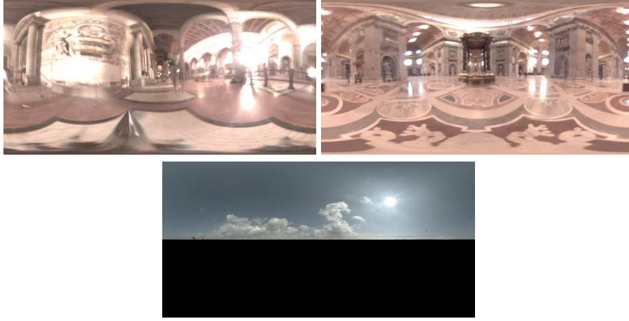
Fig. 3. The tested light probes. Top row: Galileo’s tomb in Florence, Italy, and St. Peter’s Cathedral, Rome, Italy. Both acquired from [10]. Bottom: Outdoor daylight scene. Everything below the horizon has been set to zero, so the light probe only accounts for the sun and the sky, not the ground. All probes are available via [10].
