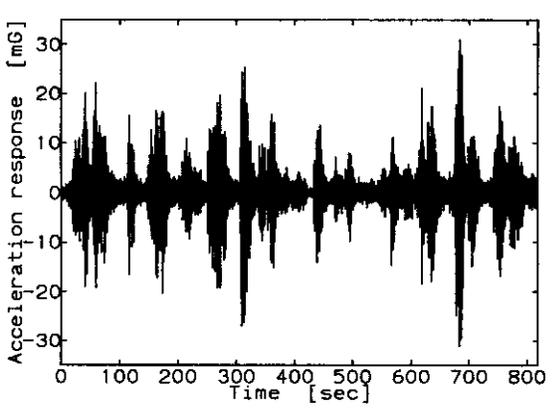
Figure 1: Typical acceleration response of the bridge.
