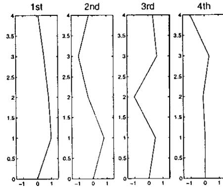
Figure 1: Mode shapes of 4 DOF system.
