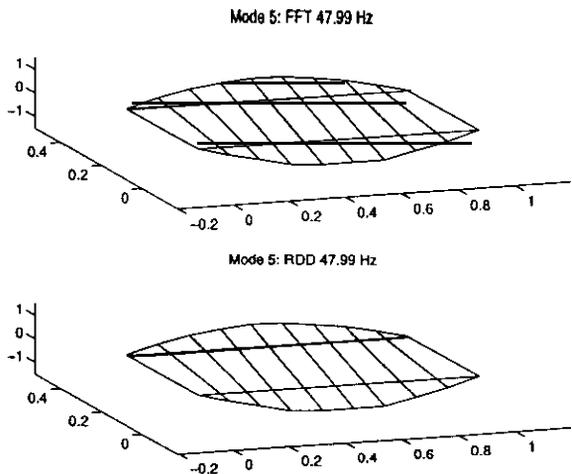
Figure 9: Fifth mode estimated using FFT and RDD-FFT.  $MAC=0.9993$
