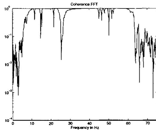
Figure 4: Typical coherence function estimated using pure FFT.
