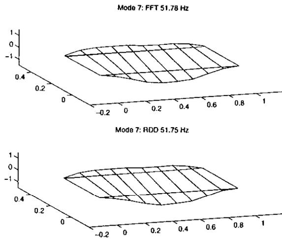
Figure 10: Seventh mode estimated using FFT and RDD-FFT.  $MAC=0.9963$ .
