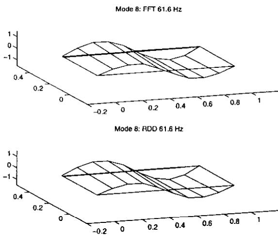
Figure 11: Eighth mode estimated using FFT and RDD-FFT.  $MAC=0.9983$ .
