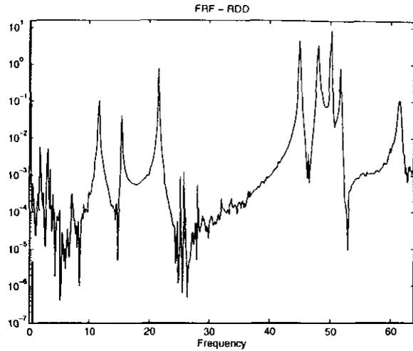
Figure 3: Typical FRF,  $|H(\omega)|^2$ , estimated using RDD-FFT.
