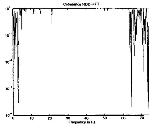
Figure 5: Typical coherence function estimated using RDD-FFT.
