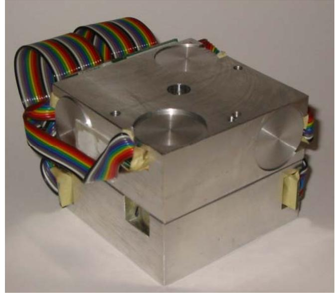
**Figure 1.** The WL 380 sensor block with 6 sensors in the dual coordinate system configuration. Left, schematic, right, photo of the sensor block, lower part of the sensor block correspond to  $x_1, y_1, z_1$ , upper part to  $x_2, y_2, z_2$ .
