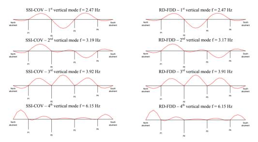
Figure 7 Identified frequencies and mode shapes
