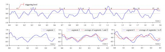
Figure 2 Basic concept of the RD technique
