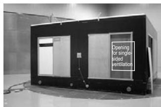
Figure 3. The building in the wind tunnel at BRI (left) and the dimensions (in mm) of the building (right).
