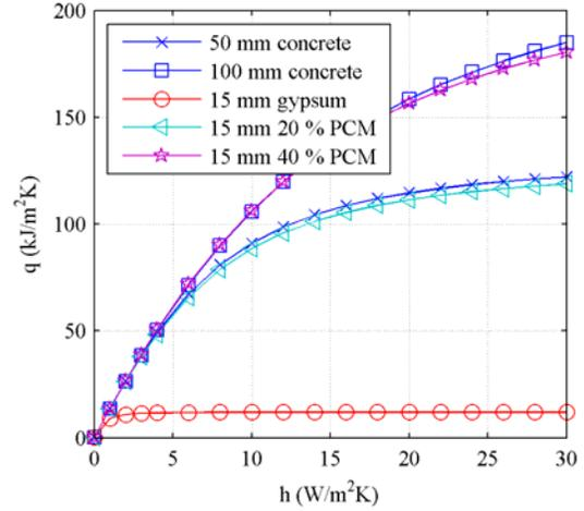
Figure 6: Effect of integrated PCM on the diurnal heat storage capacity,  $q$  depending on the heat transfer coefficient,  $h$ . Gypsum plaster board with different PCM contents compared to concrete slabs.
