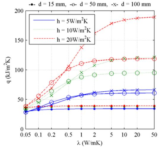
Figure 5: Diurnal heat storage capacity,  $q$  depending on the thermal conductivity,  $\lambda$  for different heat transfer coefficients,  $h$  and slab thicknesses,  $d$ ;  $\rho c = 2.6 \text{ MJ/m}^3\text{K}$ .
