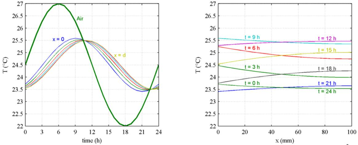
Figure 1: Temperature profile in a 100 mm thick concrete slab with convective boundary condition ( $h = 10 \text{ W/m}^2\text{K}$ ), exposed to a sinusoidal air temperature ( $24.5 \pm 2.5 \text{ }^\circ\text{C}$ ) on one side ( $x = 0$ ) and adiabatic boundary condition on the other side ( $x = 100 \text{ mm}$ ). Temporal profile at different layers of the slab,  $\Delta x = 20 \text{ mm}$  (left) and spatial profile at different time-steps,  $\Delta t = 3 \text{ h}$  (right).
