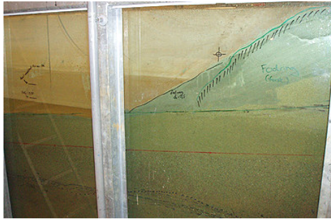
Figure 6. Profile of the beach before (left) and after (right) the test, (Holmgren et al. 2006a).
