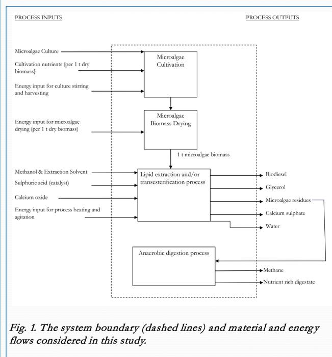
Fig. 1. The system boundary (dashed lines) and material and energy flows considered in this study.
