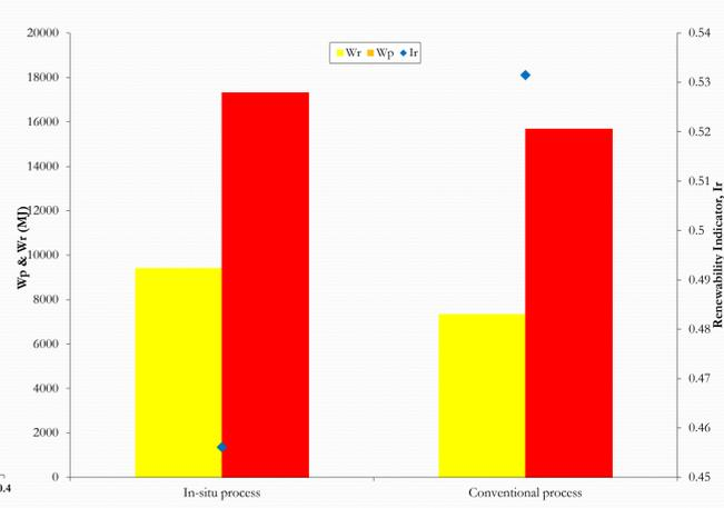
Fig. 4. Comparison of the renewability indicators for biodiesel production integrated with CH<sub>4</sub> recovery from the microalgae residues
