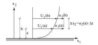
Figure 5.14: Production of turbulent kinetic energy.
