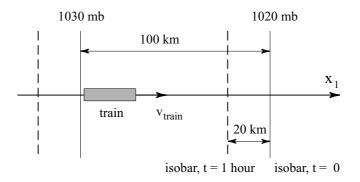
Figure 1.6: Rate of change of pressure in a train.
