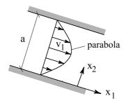
Figure 2.8: Velocity profile in Poiseuille-flow.
