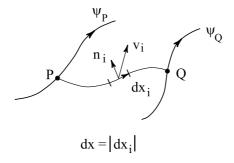
Figure 1.27: Integration path between two streamlines.
