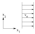
Figure 1.26: Velocity profile in uniform flow.
