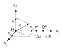
Figure 1.23: Calculation of the velocity at point Q.
