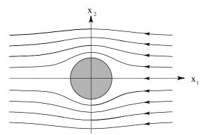
Figure 3.6: Two-dimensional potential flow around a circular cylinder.
