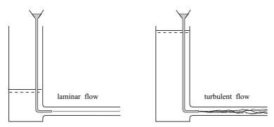
Figure 1.5: Laminar and turbulent flow.
