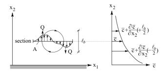
Figure 8.2: Definition sketch, convective transport caused by fluctuations.
