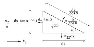
Figure 2.3: Definition sketch, stresses on a fluid body in a resting fluid.
