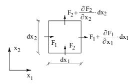
Figure 2.11: Flux of dissolved substance through a control surface.
