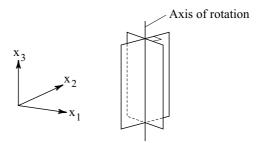
Figure 1.9: Device ("Vorticity meter") for "measurement" of the  $x_3$ -component of rot  $\vec{v}$ .
