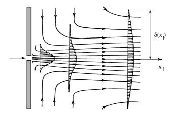
Figure 6.3: Sketch of flow in two-dimensional jet.
