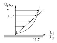
Figure 5.12: Smooth wall. Velocity profile close to wall.
