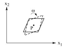
Figure 1.19: Deformation of the fluid element at P.
