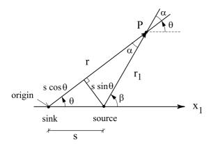
Figure 3.3: Definition sketch, two-dimensional dipole flow.
