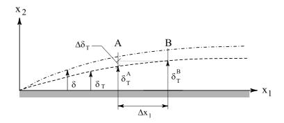
Figure 11.4: Definition sketch. Numerical calculation of thermal boundary layer
