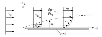
Figure 4.5: Boundary layer on a flat plate.
