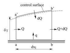
Figure 11.3: Definition sketch. Thermal boundary layer. Q is volume flux and q is the transfer of thermal energy from plate to fluid.
