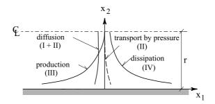
Figure 5.15: Energy balance of turbulent energy,  $\overline{k}$ , in a pipe flow. Roman numerals refer to the terms of equation (7.14).
