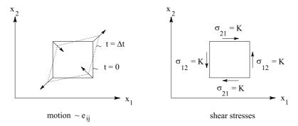
Figure 2.6: Deformations and shear stresses in Couette-flow.
