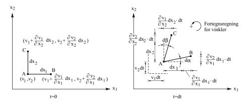
Figure 1.8: Angular motions of line segments in a velocity field.
