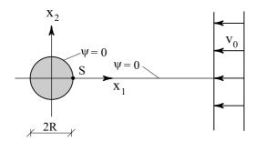
Figure 3.5: Definition sketch. Two-dimensional flow around a cylinder.
