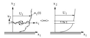
Figure 5.8: Dynamically equivalent descriptions of turbulent flow.
