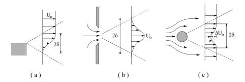
Figure 6.2: Three types of free turbulence: (a) mixing layer, (b) submerged jet, (c) wake behind a body
