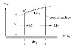
Figure 4.4: Control surface for boundary layer flow.
