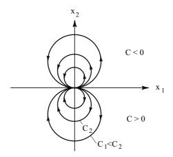
Figure 3.4: Streamlines, two-dimensional dipole flow.
