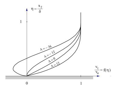
Figure 4.6: Non-similar velocity profiles in boundary layers.
