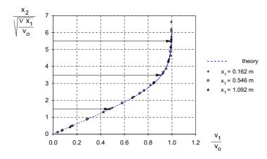
Figure 4.2: Velocity profiles in air flow along a plate corresponding to  $v_o = 10$  m/s and  $\nu = 15 \cdot 10^{-5}$  m<sup>2</sup>/s.
