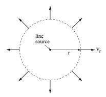
Figure 3.2: Velocity field at a line source.
