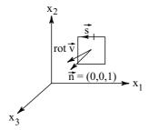
Figure 1.11: Usage of Stokes's theorem to calculate (rot  $\vec{v}$ )<sub>3</sub>.
