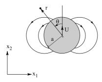
Figure 3.13: Streamlines seen from a coordinate system fixed in space.
