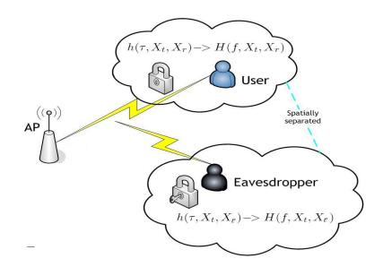
Figure 1.2: Difference between user and eavesdropper [1]
