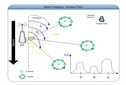
Figure 1.5: Beam Hopping applied by AP
