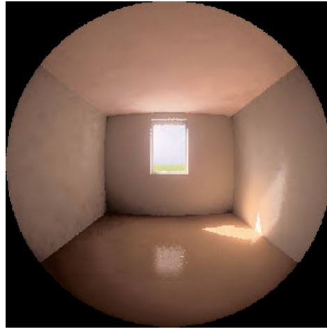
Figure 25. Fish eye rendering for the vertical window in April at 10:00 hours.
