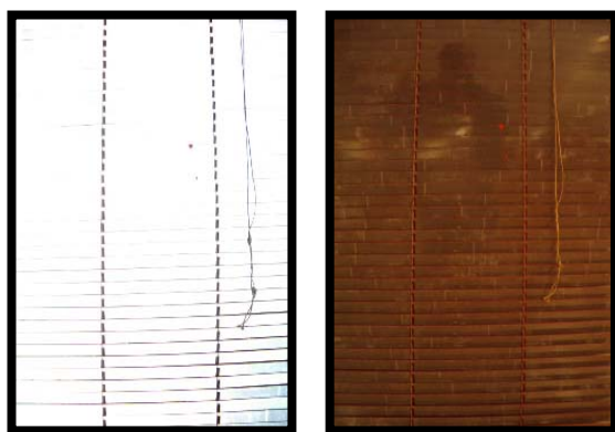
Figure 9. Retroreflective microprisms window blind
