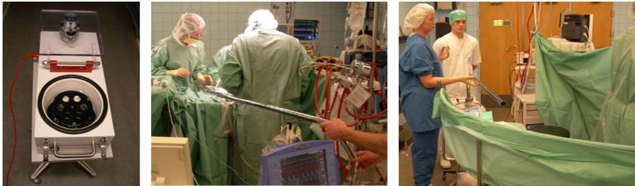
Figure 5. Left: Slit sampler Biap CDII applied for bacteria measurements during the operations. Centre and Right: Operation of slit sampler using extension pipes.
